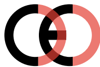
False CE Mark (too close)
